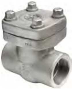
SSCK800 SWING CHECK VALVE API602 316 Stainless Steel Stellite seat CLASS 800 (2000psi) NPT or socket weld 15mm to 50mm
