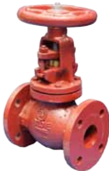
B201E CAST IRON GLOBE VALVE Outside Screw and Yoke Bronze seat Flanged AS2129 Table E 50mm to 300mm
