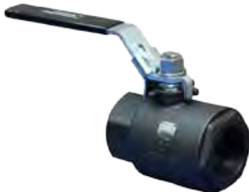
BL3000 BALL VALVE NPT 3000psi WCB 2PCE PEEK seats Firesafe Certified, Full bore Lever operated 8mm to 50mm
