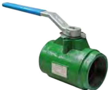
QZ602 1000PSI BALL VALVE NPT DUCTILE IRON RPTFE seats 100mm
