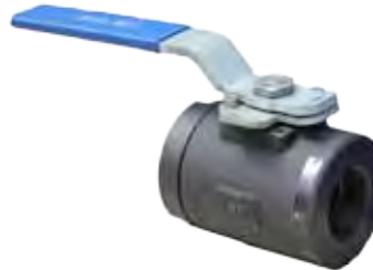
BL1500 BALL VALVE NPT CLASS 1500 (3700psi) A105N 2PCE CTFE seats Firesafe Certified, Full bore Lever operated 15mm to 50mm
