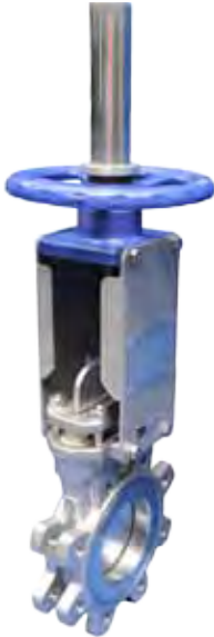
BKGV-A LUGGED ANSI 150 LB KNIFE GATE 316 Stainless Steel EPDM or METAL seat 1000Kpa 50mm to 600mm
