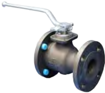
ZRB 1 PIECE FLANGED ANSI 150/300 BALL VALVE A216 WCC Reduced bore PTFE seats 15mm to 250mm Firesafe Certified API 607
