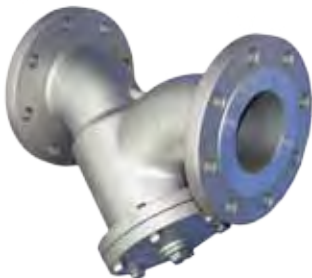
YST-150 FLANGED Y STRAINER ANSI 150 316 Stainless Steel Integral drain plug 15mm to 300mm Available undrilled
