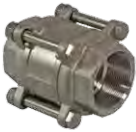
V3WC THREE PIECE CHECK VALVE 316 Stainless Steel Spring loaded 40 BAR 10mm to 100mm BSP
