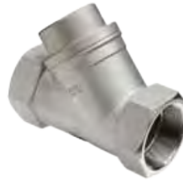
VPC PISTON CHECK VALVE 316 Stainless Steel Inclined PTFE seat 40 Bar Female BSP 8mm to 50mm
