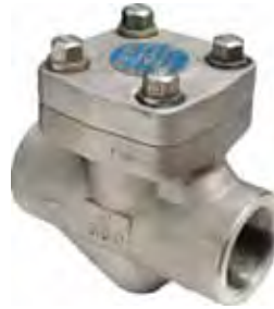
SSCP800 PISTON CHECK VALVE API602 316 Stainless Steel Stellite seat CLASS 800 (2000psi) NPT or socket weld 15mm to 50mm
