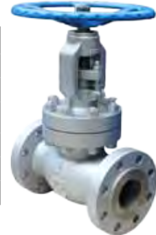
SSGL-150/300 FLANGED GLOBE VALVE ANSI 150 or ANSI 300 316 Body, STELLITE seat OS&Y Graphite Packing Spiral Wound Gasket 15mm to 300mm
