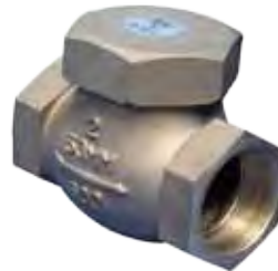
B521 PISTON CHECK VALVE Bronze for Steam 410ss seat. Union Cover. 300PSI 15mm to 50mm BSPT
