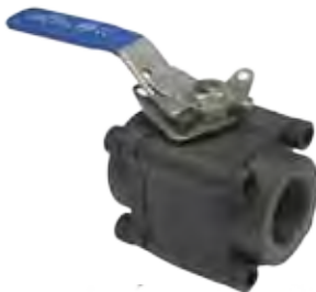
BL800 BALL VALVE API 602 A105N CLASS 800 (2000psi) Full bore Firesafe Certified 15mm to 50mm Available in NPT or socket weld
